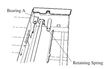
Figure 5.5 Move the Retaining spring
